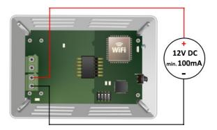
Important: If a wired remote controller of the AC manufacturer is connected in the same bus, communication may shut down. In case it happens, use an external power supply connected to the PS connector in our device to overcome this situation.
