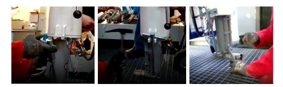
✓ Insert the pump-mixing spiral
