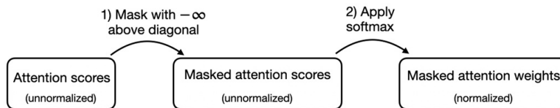
Figure 3.21 A more efficient way to obtain the masked attention weight matrix in causal attention is to mask the attention scores with negative infinity values before applying the softmax function.
