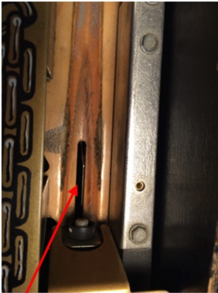
Switch which is active when a ball is resting in the lane.
